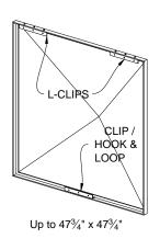
5. Peel off the back of the Hook & Loop to expose the adhesive. Press the diffuser to the wall above the wall brackets and slide the diffuser onto the wall brackets while holding the bottom of the diffuser slightly away from the wall. With the L-Clips engaged, level and adjust the position. Once the desired positioned is achieved, press the bottom of the diffuser firmly to the wall to adhere the hook & loop.
